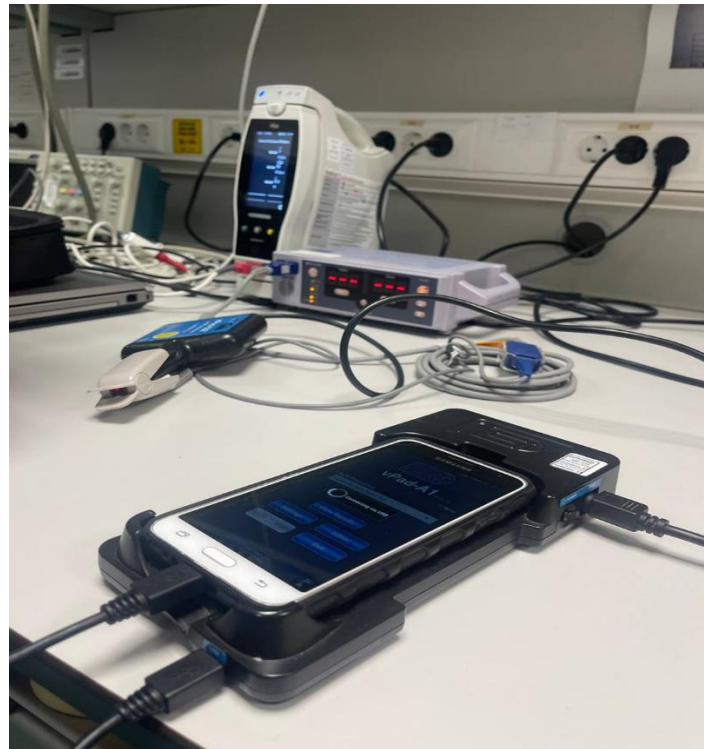
Figure 10. Pulse Oxymetry Analyzer
