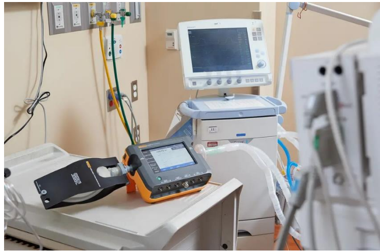
Figure 5. Gas flow analyzer
