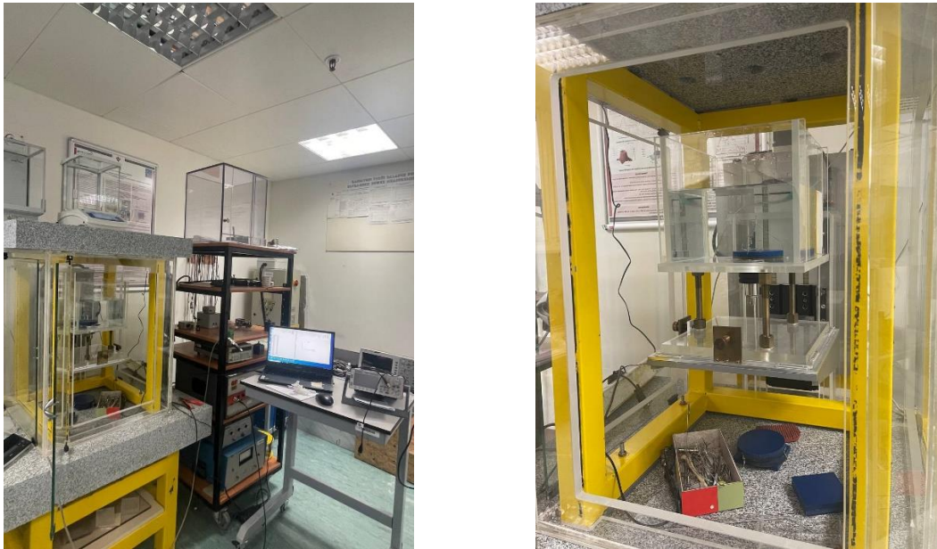
Figure 1. Ultrasonic power measurement device
